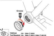
Tool compatible with torque wrench
